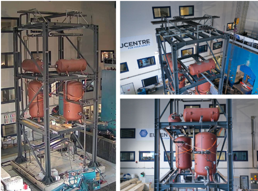
Figure 4.14: Case study #2: Mock-up photographs at the EUCENTRE Laboratory (after Butenweg et al 2020, [43]).
