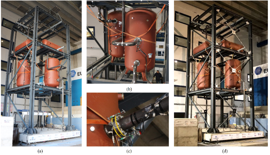
Figure 5.1: Photos of the SPIF's mock-up @EUCENTRE, Pavia: a) the MRF configuration; b) the two installed vertical tanks; c) details of the BFJ between vertical tank and piping system at 1 st level; d) the BF configuration.
