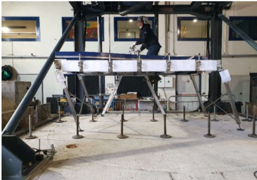
Figure 2.21: Collapse of the supporting system of the conveyor at base level for record TH #8-110% .
